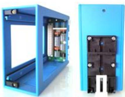
The connection board with FI32 female multi-point connector can also be installed in table-tops or 19" racks. For Ex applications, the connection boards are different (female multi-point connectors are coded).
